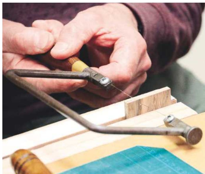
Waste is cut away in the normal manner, using a fret saw
